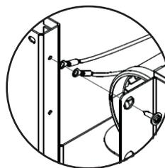
The fan can be removed for cleaning by unscrewing the locating screws. Remember to disconnect the power supply before touching the fan.
