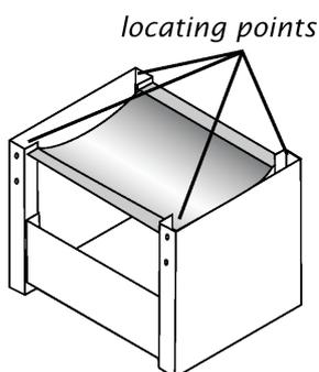
You must now attach the firebox. Lay the firebox on its back. Locate the column onto the four locating points on the base of the heater. Ensure the side of the column with a 45 mm gap on the bottom edge goes at the rear of the heater.
